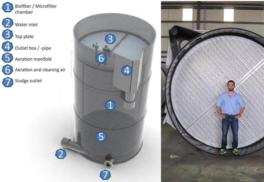
*Normally PE biofilters are placed above ground level and fitted with a sludge discharge valve for easy flushing and cleaning. The sludge water is lead to the wastewater treatment system outside the aquaculture recirculation system. The picture on the right reveals the size of a large PE biofilter. Source: AKVA group.*
