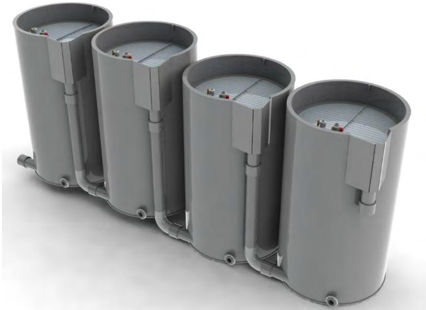
*Most of the organic material is removed by heterotrophic bacteria in the first chamber. The consequent low organic load in the latter chambers secures a thin nitrifying biofilm for converting ammonia to nitrate. The last chamber is called a microparticle filter and is designed for removal of very fine particles that have not been removed by the mechanical filter. This type of filter can also be created in concrete.*
