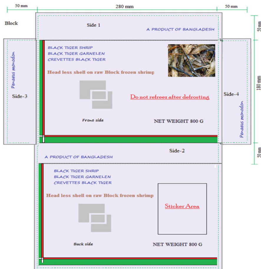
Fig. 8.6 Dimension and design of inner box for block products
