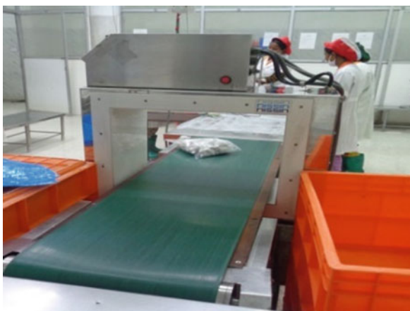
Fig. 8.30 Metal detection of shrimp
