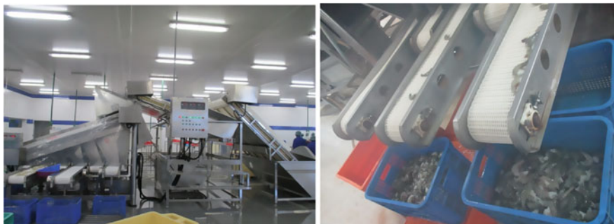
Fig. 2.52 Grading of shrimp with automatic grading machine
