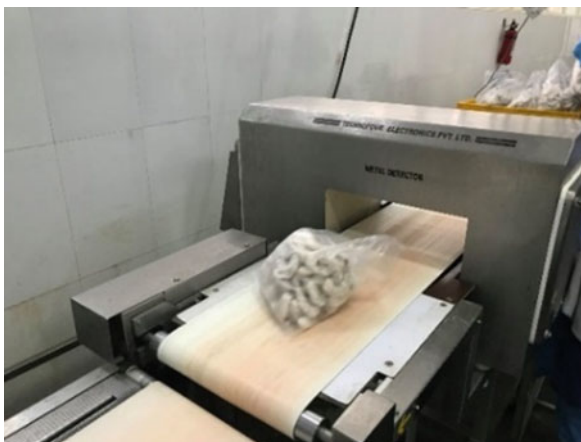
Fig. 8.31 Metal detection of shrimp
