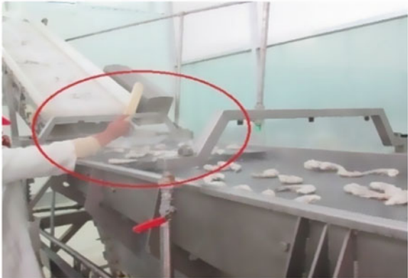
Fig. 14.3 Hammering on clumps to remove clumps
